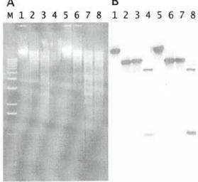
Agarose gel electrophoresis and Southern blot analysis comparing genomic DNA from yeast purified by phenol/chloroform and by ProCipitate™.
